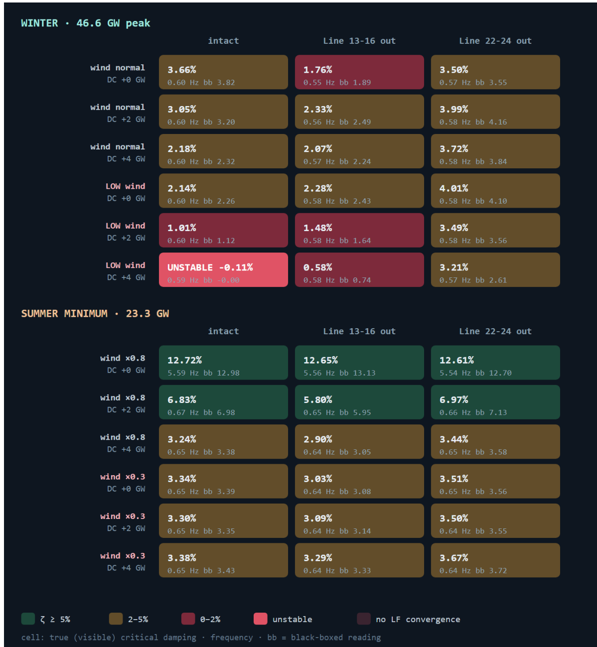
Figure 8 — The severity matrix: true critical damping per case (bb = black-boxed reading). Winter degrades toward the low-wind + DC corner; summer sits higher but data-centre growth pulls it back toward winter-like behaviour.
