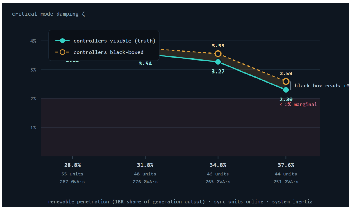
Figure 3 — Critical-mode damping vs renewable penetration at winter peak; the shaded band is the black-box optimism.
